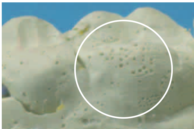
Stone Model with Hydrogen Evolution Voids
